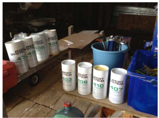
West System Epoxy used to patch hull damage where possible.
