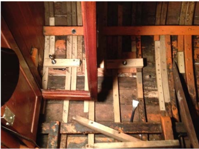
Multiple new ribs installed with hand driven brass rivets and washers
