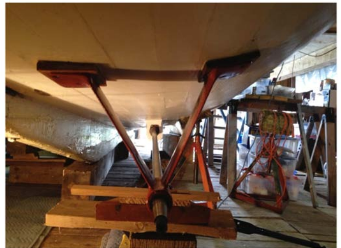
Once the shaft is perfectly aligned and in the correct position, it can be supported by the shaft struts.
