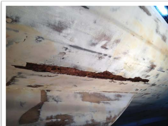
Hull damage in 90 year old planks
