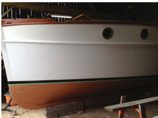
Finishing paint touches - water line corrected and repainted.
