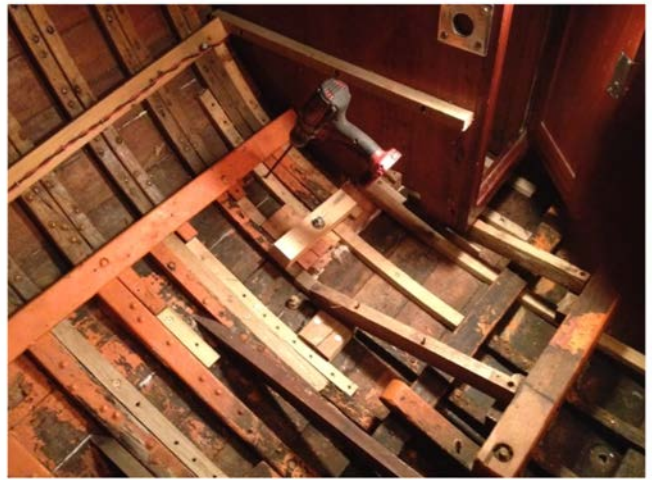
Drilling the hundreds of rivet holes
