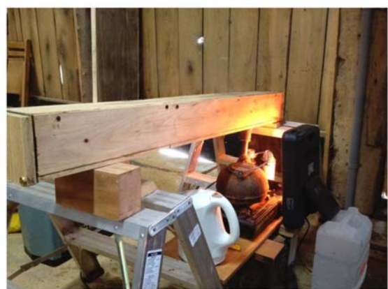
Homemade steaming box to steam and shape the Black Locust lumber into new ribs.
