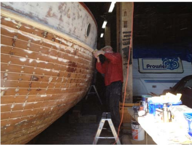
The big process of sanding and repairing the hull. Brian Tannahill sanding and sanding and sanding and sanding...
