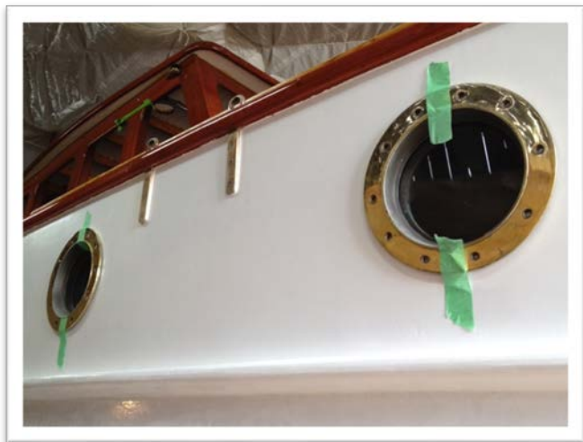
Original portholes repaired, polished, and reinstalled.
