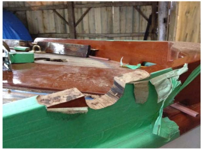
Installing the original line chocks into the new bow rebuild.
