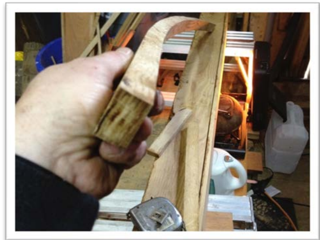
The shape of a new Black Locust rib. The Black Locust trees were sourced from Cam Graham's own property in Leith.
