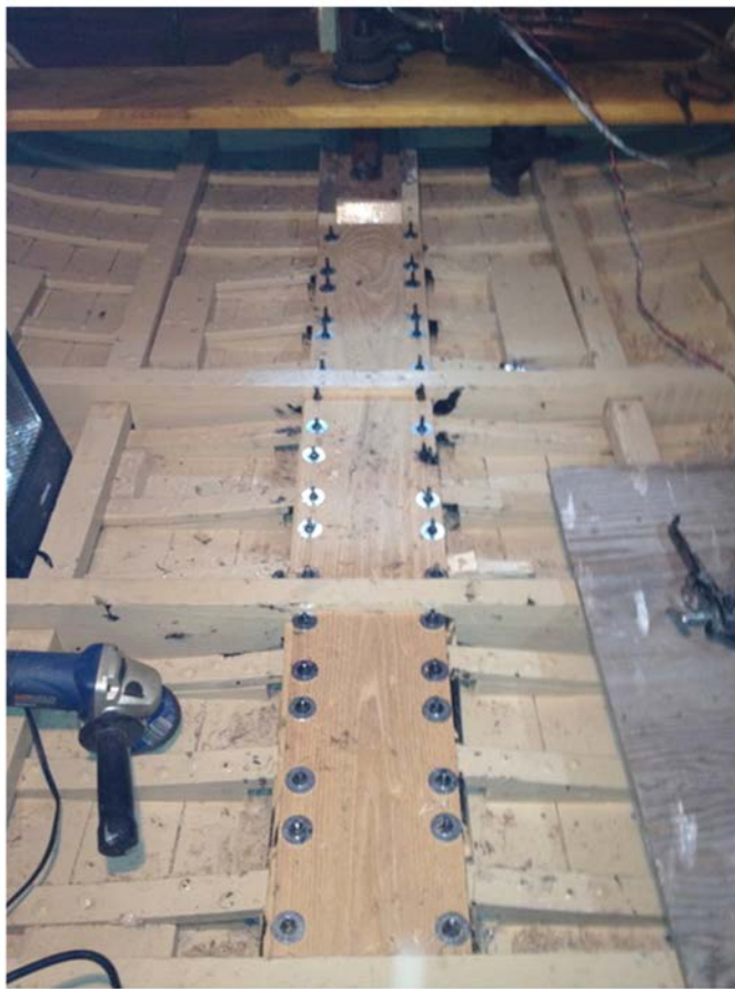
This is the biggest part of the preservation of Dragonfly. The spine of the craft was collapsing under its own weight. This was my solution to reinforcing and rebuilding the existing spine to save the Dragonfly
