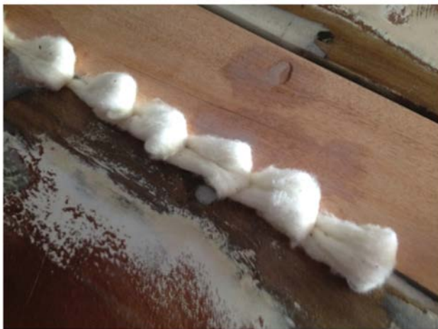
Learning cotton caulking to seal the new hull planks.
