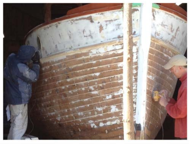
Blending the old and new planks and bow sprit with more sanding
