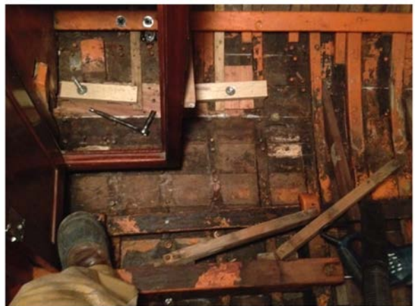
Reinstalling the bilge keels that run up either side of Dragonfly.
